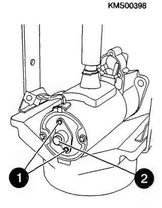
Disassembling commutator end shield
